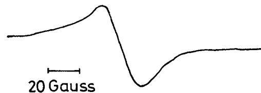
Fig. 14. ESR signal of polybutadiene irradiated with a high pressure Hg lamp at -70^{\circ}\text{C} .
