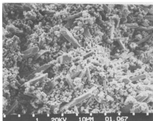
Fig. 3. Scanning electron micrograph of "precharged" positive plate made with 30% TTB and 70% Eagle-Picher (medium cure) lead dioxide prior to exposure to sulfuric acid.
