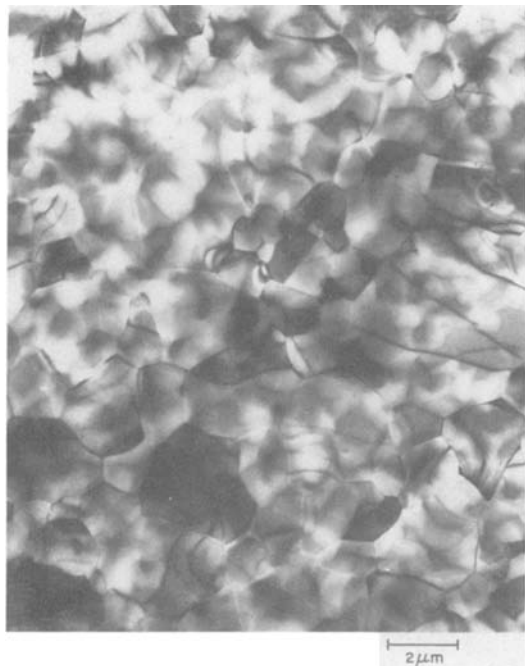
Fig. 8. TEM horizontal cross-section micrograph of LPCVD aluminum
