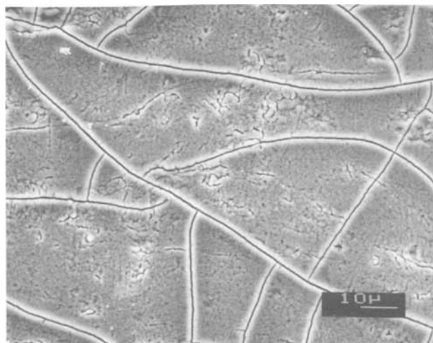
Fig. 15. a, left: SEM photo of oxide film at Ru formed thermally by decomposition of \text{RuCl}_3 coatings. b, right: Oxide film on Ru electroplated on Au. Film developed by the electrochemical cycling procedure.
