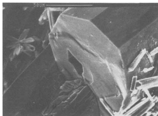
Fig. 3. Scanning electron micrograph of one end of a V 2 WO 7.5 crystal deposited onto a Pt wire at 50 mA/cm 2 under galvanostatic control. T_{melt} = 785^\circ C .
