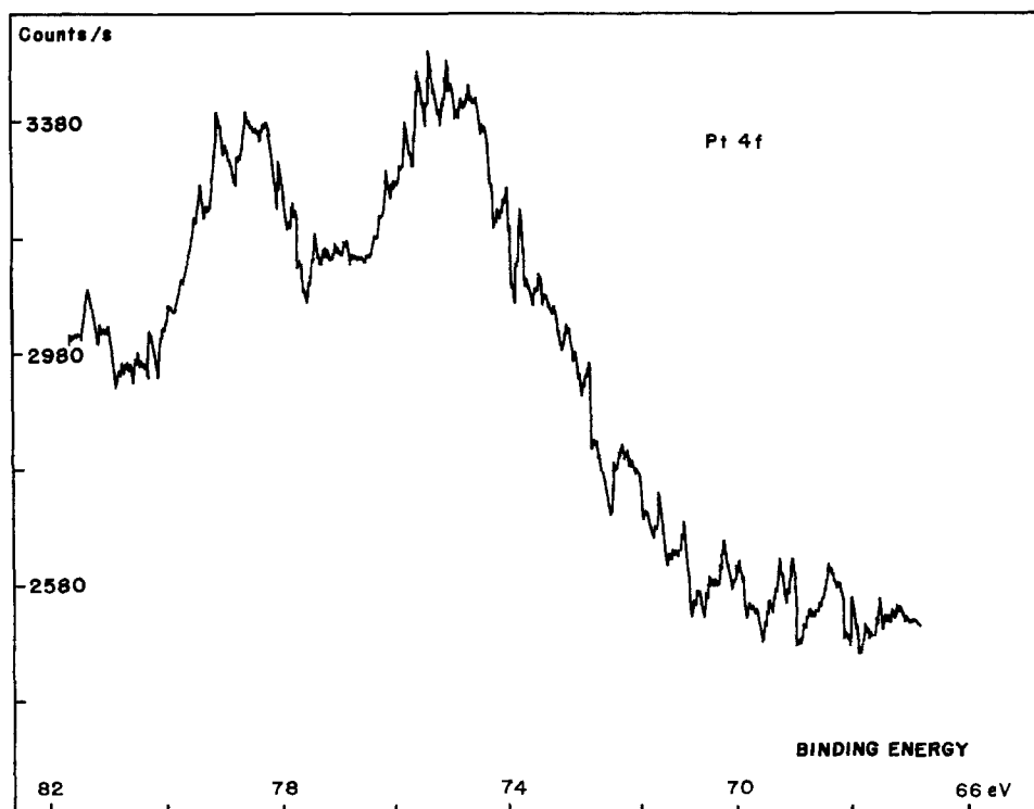
Fig. 7. XPS spectrum of the Pt 4f region for a moderately oxidized Ti sample plasma coated in a RF argon-vinylferrocene discharge with Pt foil present in the plasma reactor.
