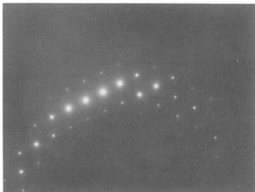
Fig. 12. A typical diffraction pattern of the recrystallized silicon.
