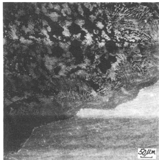
Fig. 14. The dendritic growth around a grid wire in a plate being cycled to failure.
