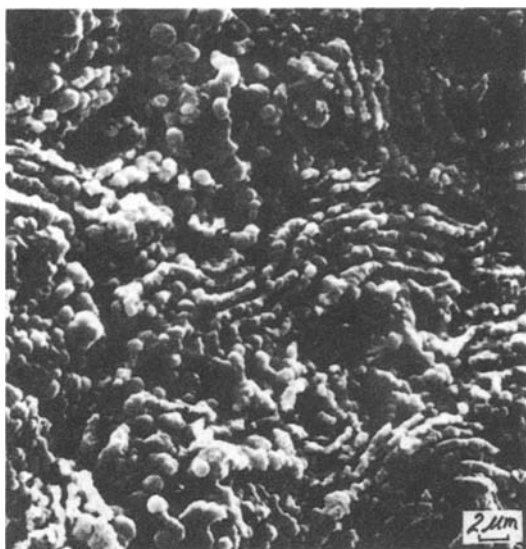
Fig. 3. Active material on the surface of an as-formed plate prepared from Fume Litharge.
