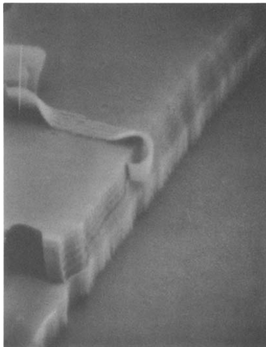
Fig. 5. SEM of a polymer film mechanically peeled away from a photoresist sidewall masking a doped polysilicon layer after etching.
