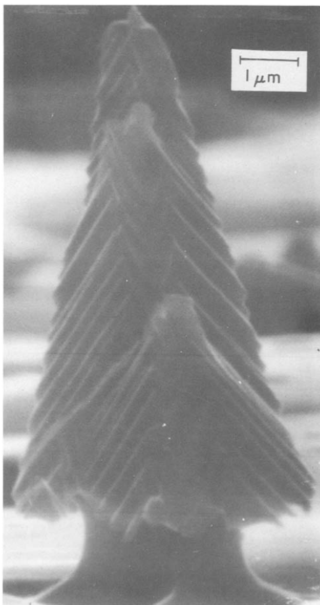
Fig. 3. SEM micrograph of a pyramidal SiO 2 growth feature formed via the reaction of O 2 with Si(100) at P(O 2 ) = 1.8 × 10 -2 torr and T s = 1090°C. The pyramid is undercut at its base via the etching reaction producing SiO.
